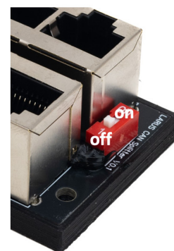
CAN termination switch CAN Splitter
