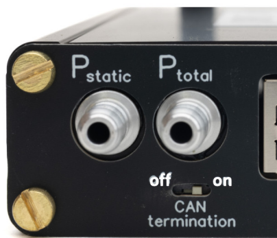
CAN termination switch LARUS Sensor Box
