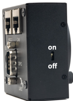
CAN termination switch LARUS Vario Display
