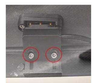
• Install the Flarm Control Box and the ACL switch in the panel according to the main manual.
