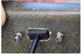
• Put the same shim of the drill template onto the panel connector. Install the panel connector (please check that **the white arrow on the black printed circuit board points towards the cockpit center**) and gently fasten the screws
