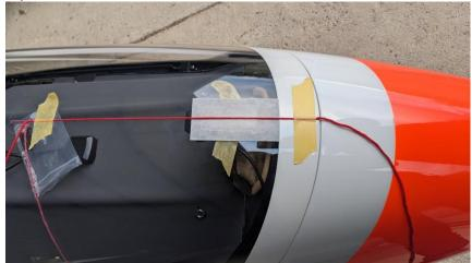
• Remove the instrument panel cover to determine the exact position of the panel cover connector
