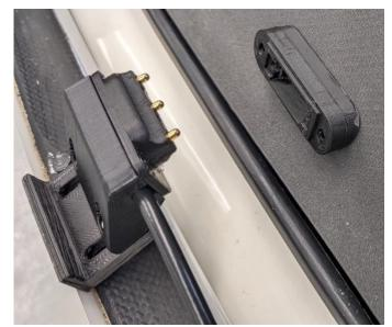
• Drill the holes for the M3 mounting screws of the opposite connector according to the drill template; drill (and file the rectangle) in the center for the cable.
